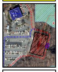
Option 06 proposes a new 65,388 sq. ft. free-standing building in the wooded area to the south-east end of the property. This option has similar benefits to Option 05 but removes the parking displacement drawback, but would require land clearing and other additional site scope. From a programmatic and phasing standpoint, this option is preferable and recommended.
